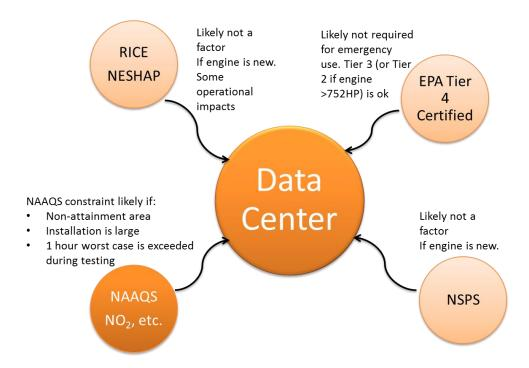
A summary Table of EPA Regulations associated with large stationary Diesel engines used in emergency applications is shown in Table 1.
